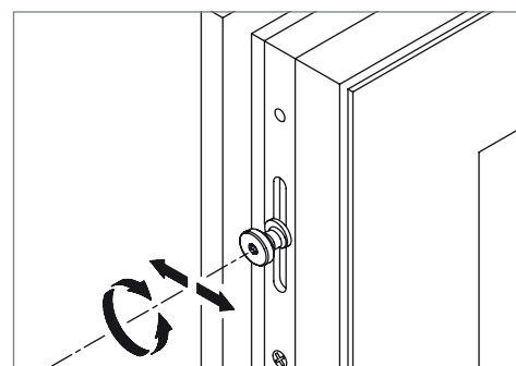
Gasket pressure adjustment – mushroom pin
